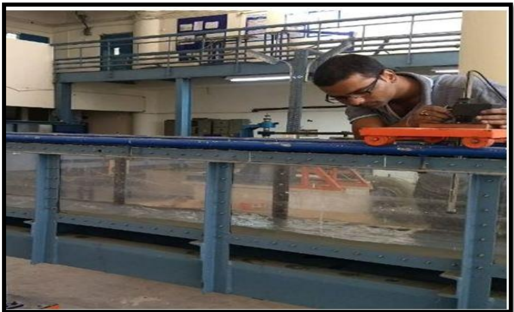
Figure 3.6: Formation of hydraulic jump on rough surface
