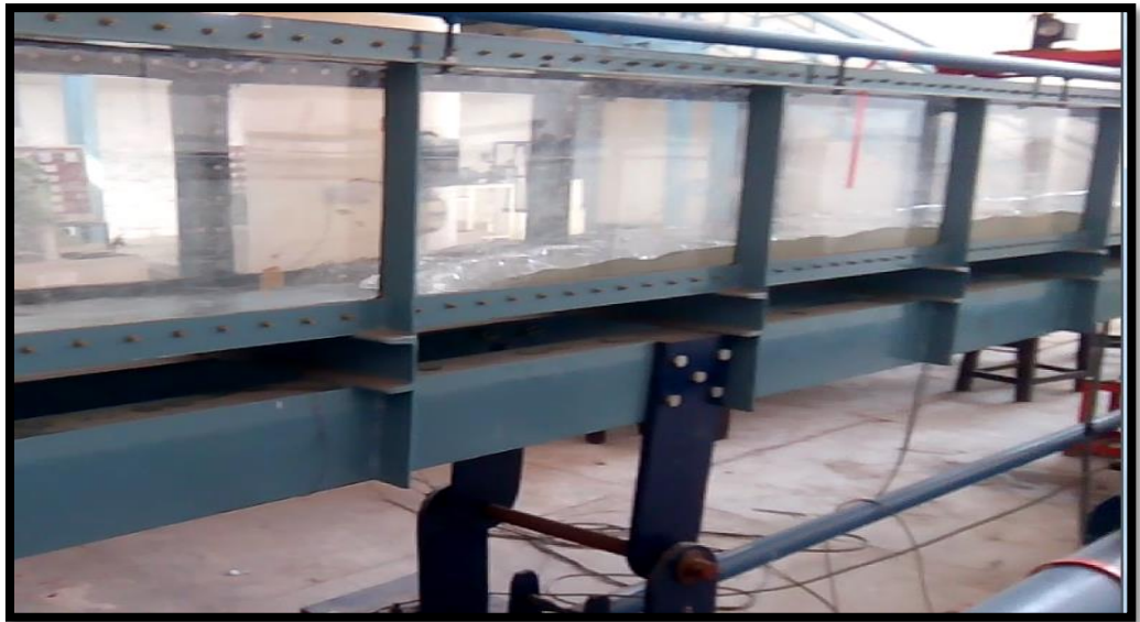
Figure 3.4: Formation of hydraulic jump on smooth surface
