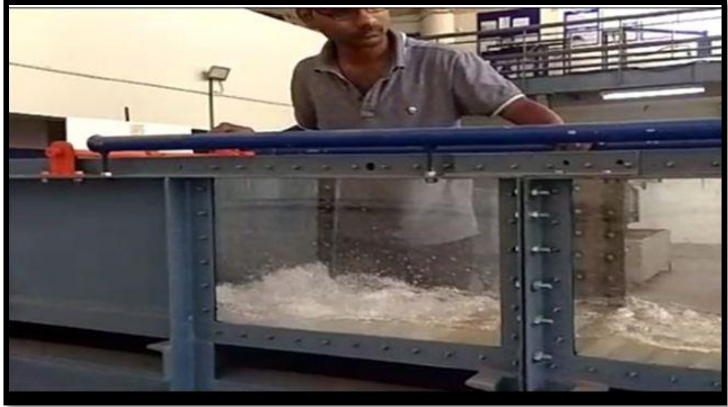
Figure 3.5: Formation of hydraulic jump on rough surface.
