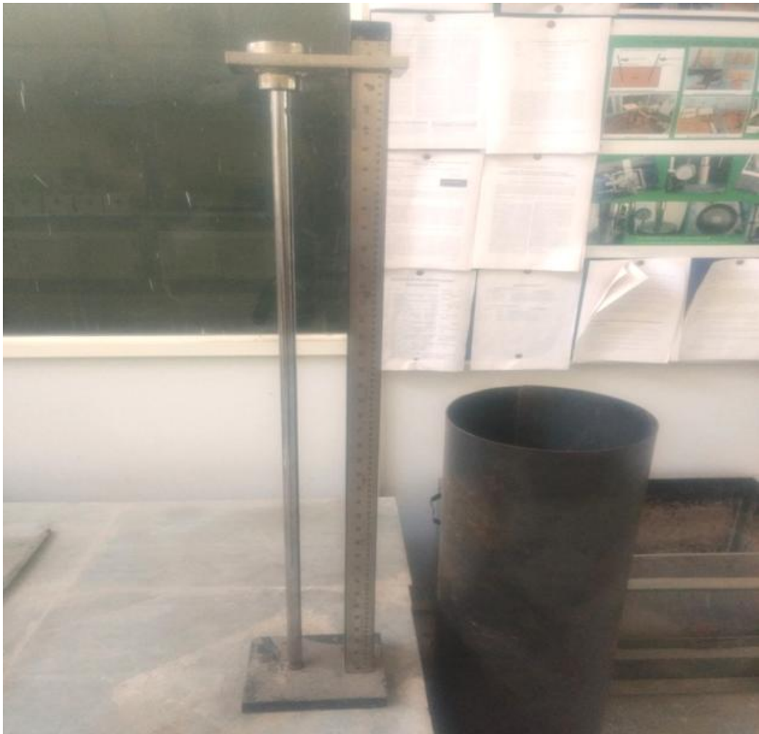
Fig. 3.7 The DCP device and the testing container.
