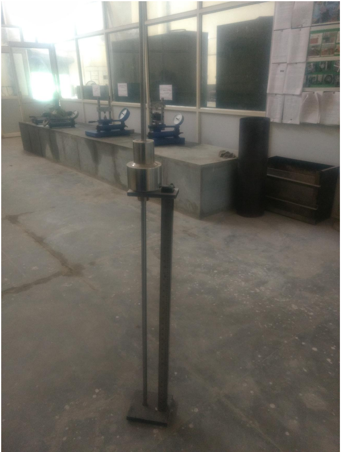
Fig. 3.5 The DCP device fully assembled.
