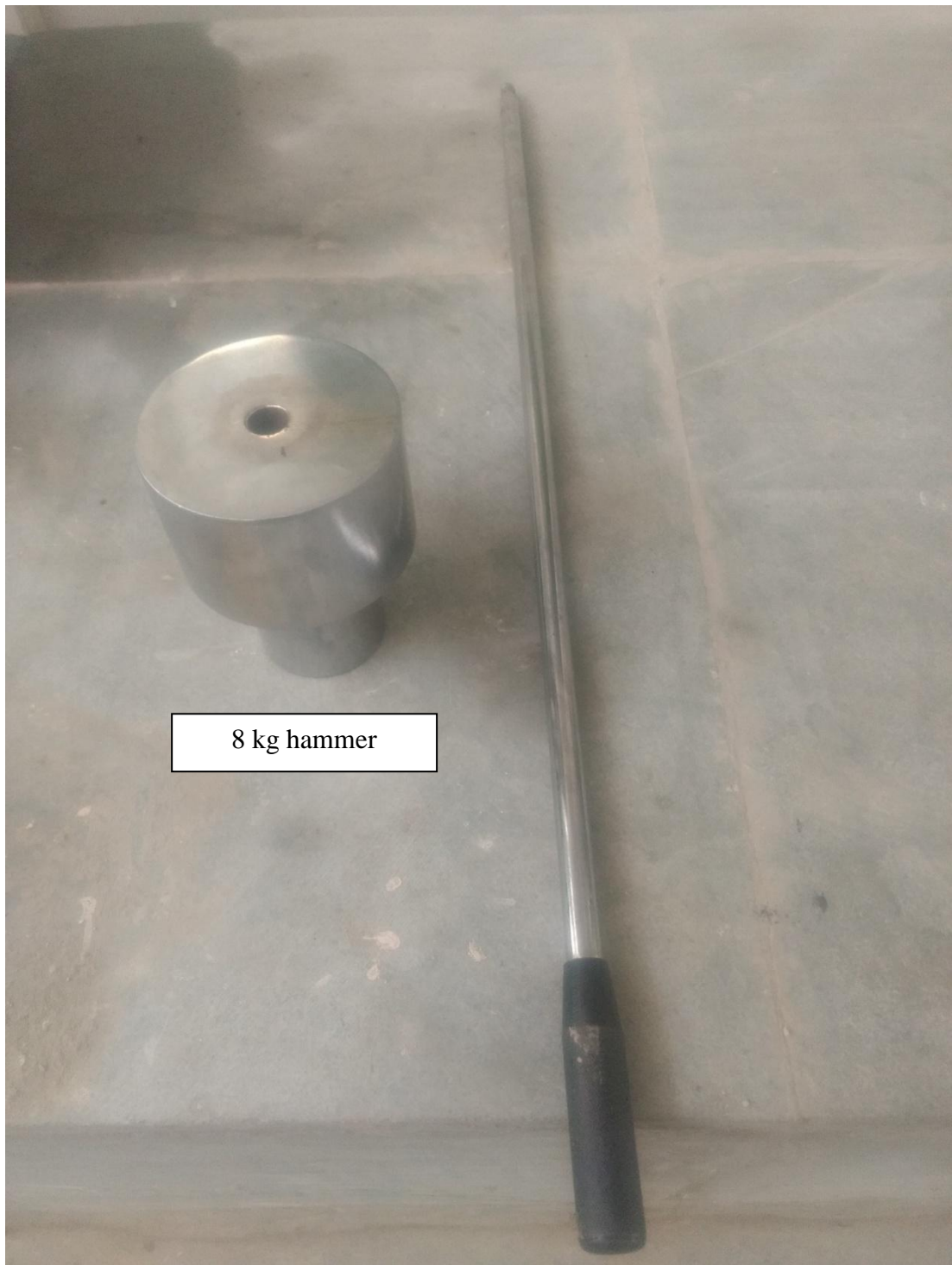
Fig. 3.6 The hammer and the sliding rod.
