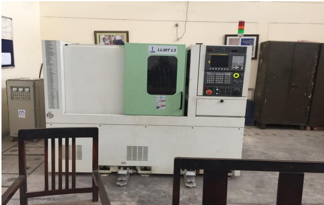
Figure 3.1 CNC Turning Machine (Type: LL20T3)
