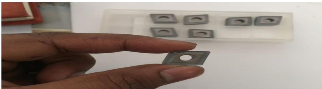
Figure: 1.5 Carbide tool material (CNMG 120408-THM-F)
