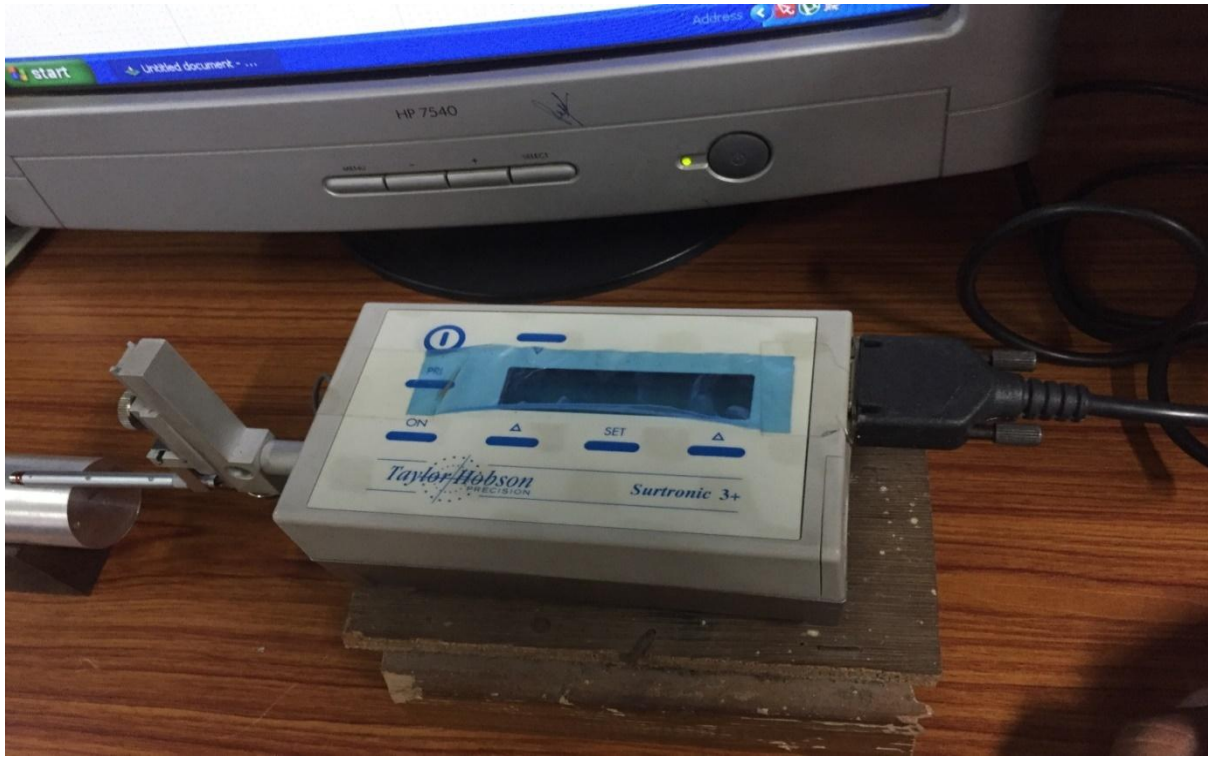
Figure: 3.2 Surface roughness measurement apparatus
