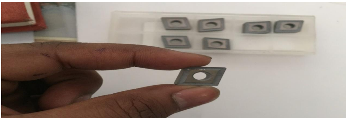
Figure: 3.10 Carbide tool material (CNMG 120408-THM-F)
