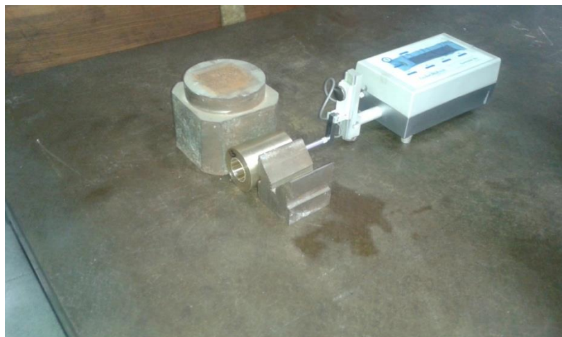
Figure 4.4: Talysurf measuring the internal surface roughness
