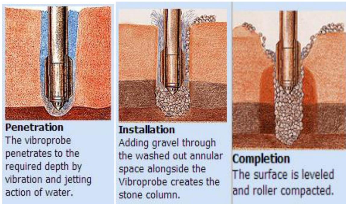
Fig. 1.3 Wet top feed method
