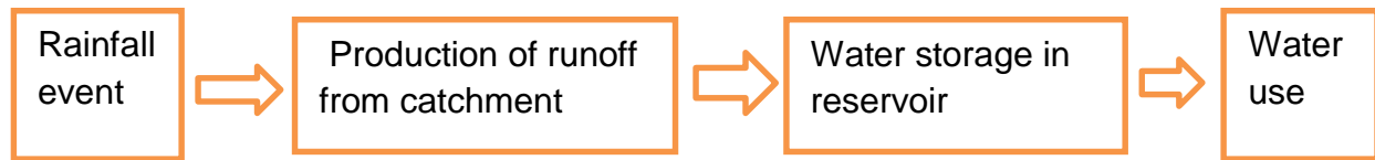
Figure 1.1 Flowchart illustrating the fundamental rainwater harvesting processes
