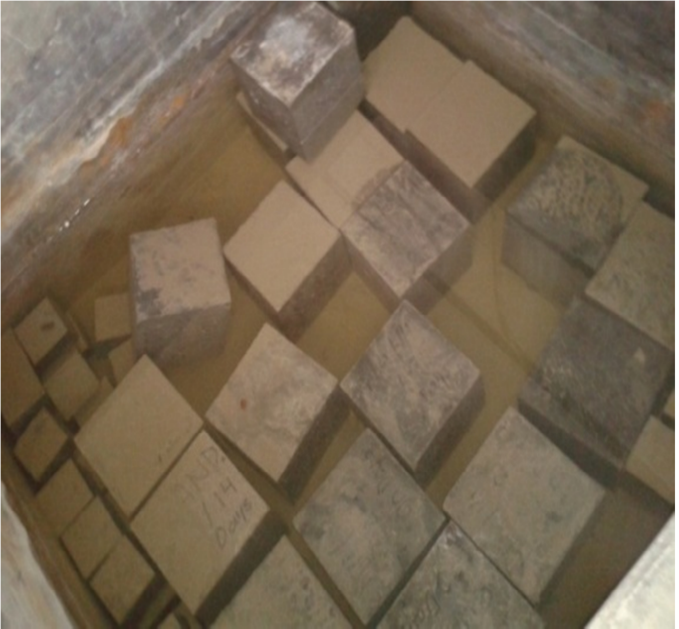
Fig. 3.3(f) Concrete cubes in curing tank
