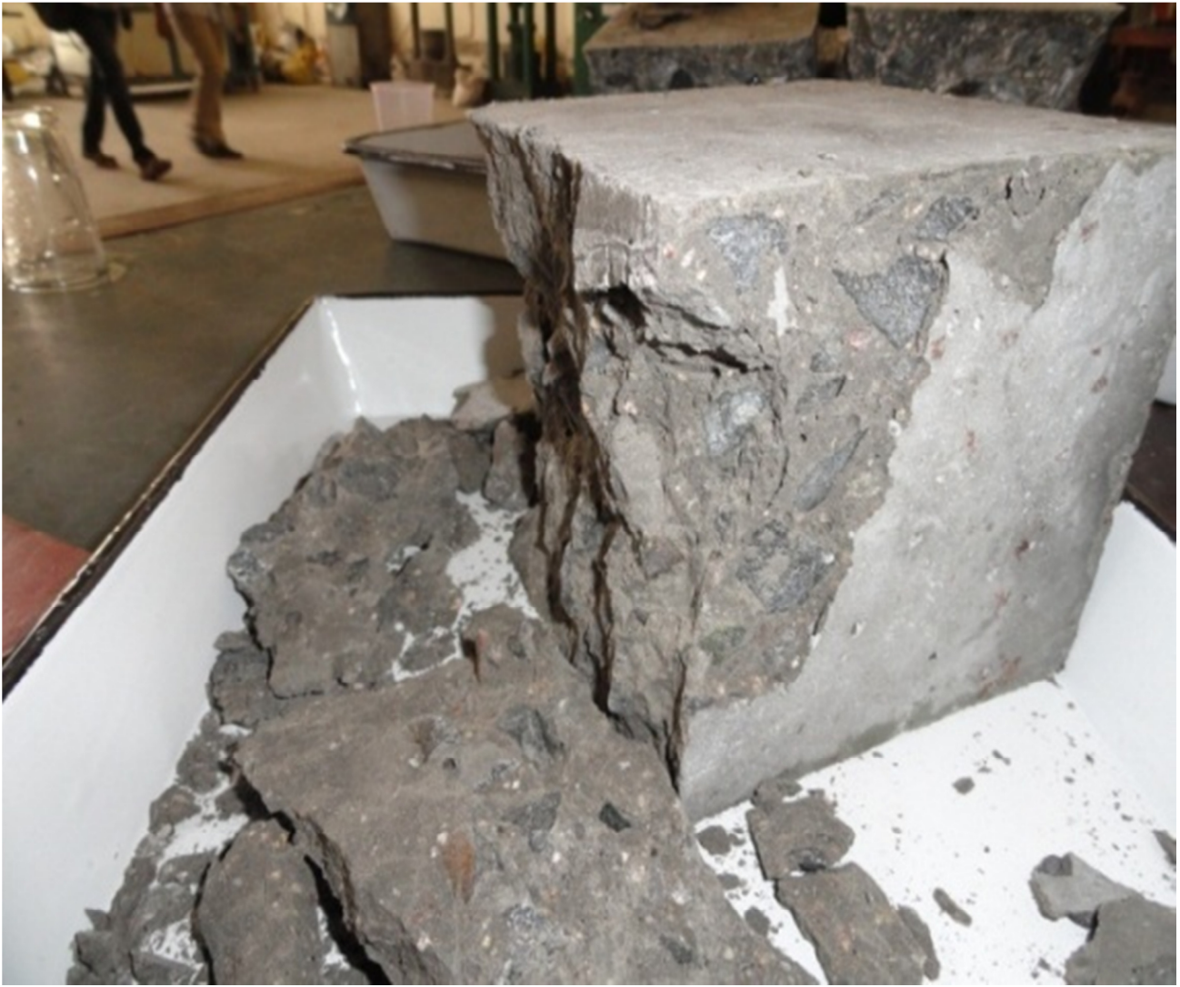
Fig 3.3(j) Plain Concrete cube under compression testing machine
