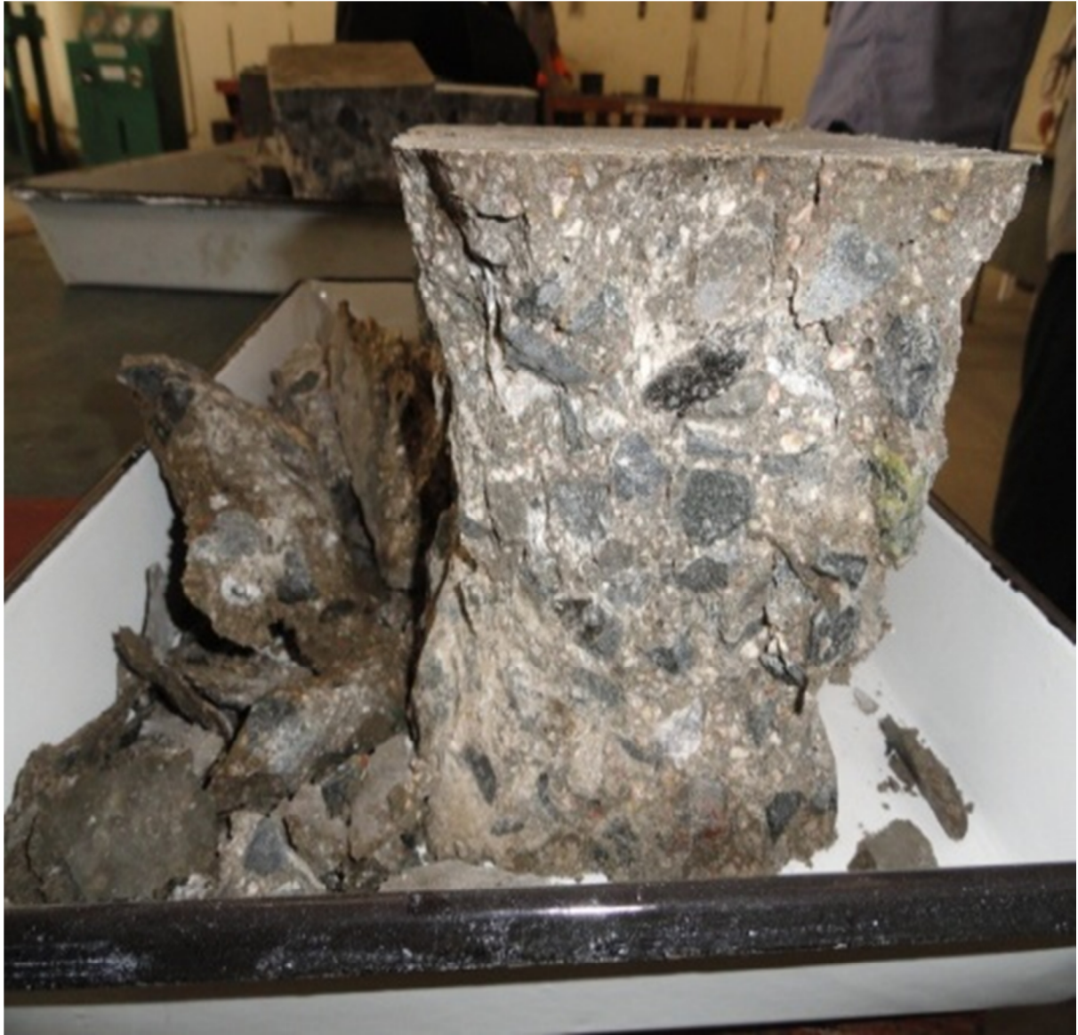
Figure 3.3(k) Fractured surfaces of flyash based concrete cubes exposed after compression.
