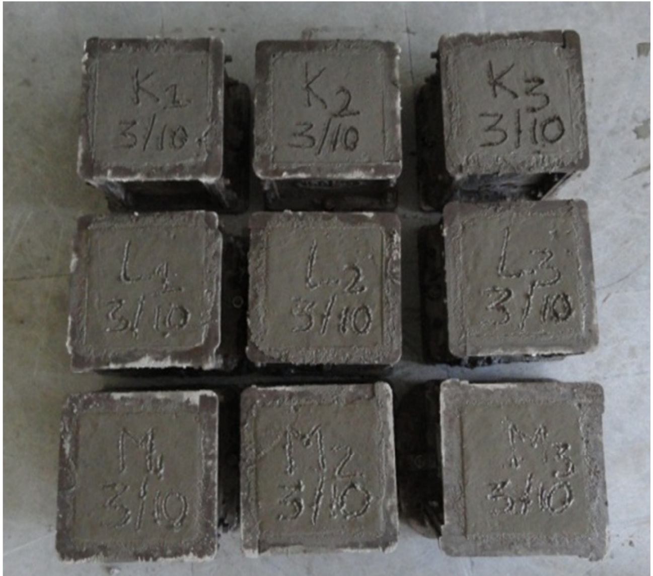
Fig 3.3(c)(i) Plain Concrete in moulds
