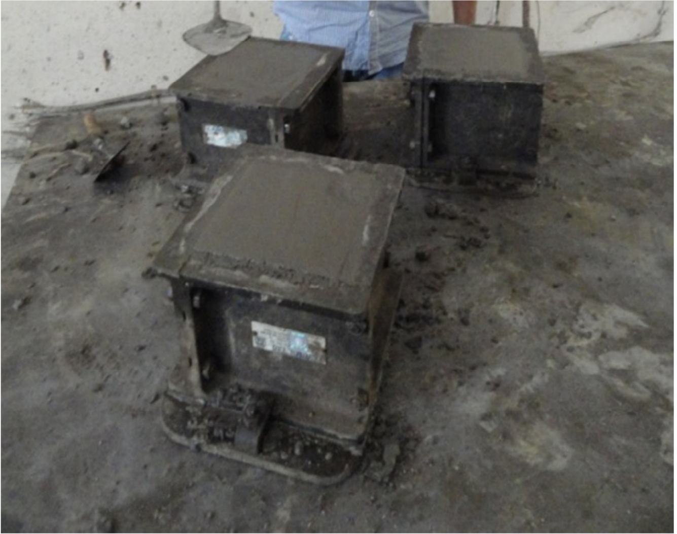
Fig.3.3(c) (ii) Flyash based concrete in moulds
