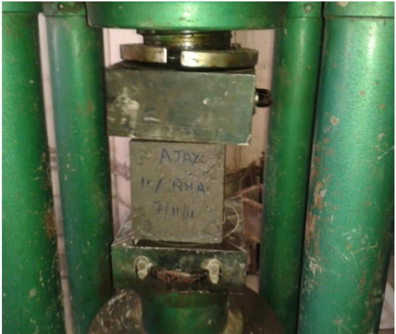
Fig.3.3(i) Concrete cube tested under compression testing machine
