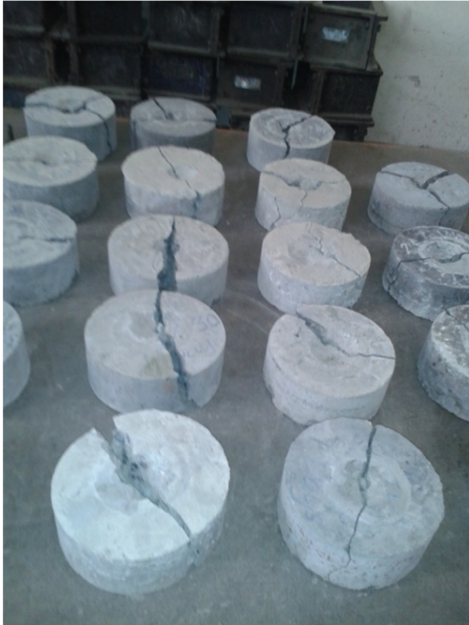
Fig 4.3(j) Concrete specimen after impact test showing the crack pattern
