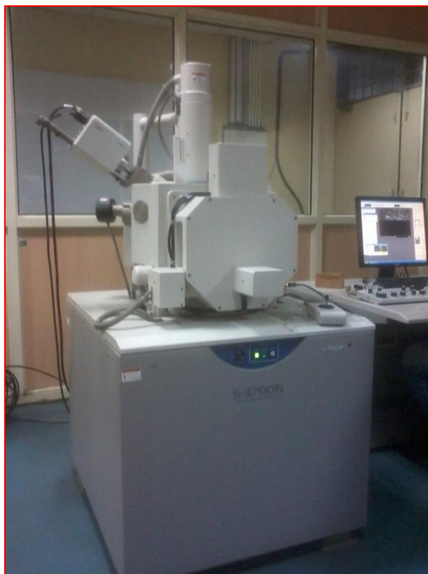
Figure 2.17: SEM HITACHI, Model No.S-3700N with EDS-X with X-ray at DTU, Delhi
