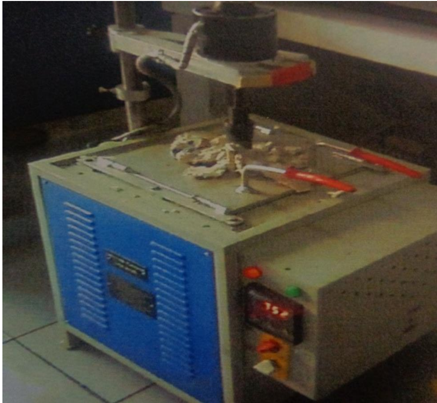
Fig. 27. Furnace used for making aluminium foam[39]
