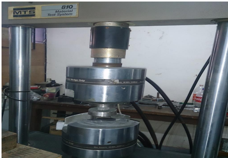
Fig. 34.MTS 810 material test system used for quasi static compression
