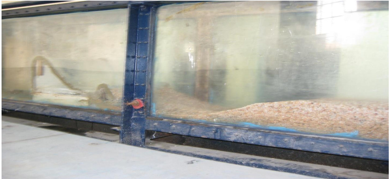
Figure 3.14: Scouring profile at downstream of ogee spillway with subsidiary dam with particle size 4.75mm on tilted bed (slope 1/300)
