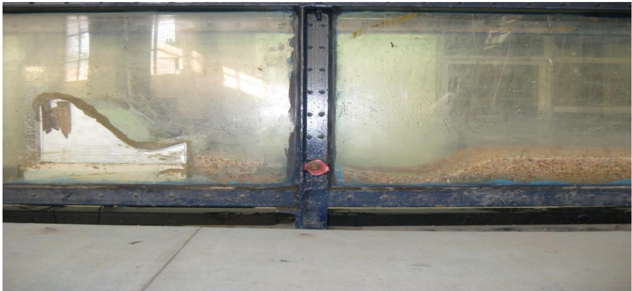
Figure 3.15: Scouring profile at downstream of ski jump bucket spillway with particle size 4.75mm on tilted bed (slope 1/300)
