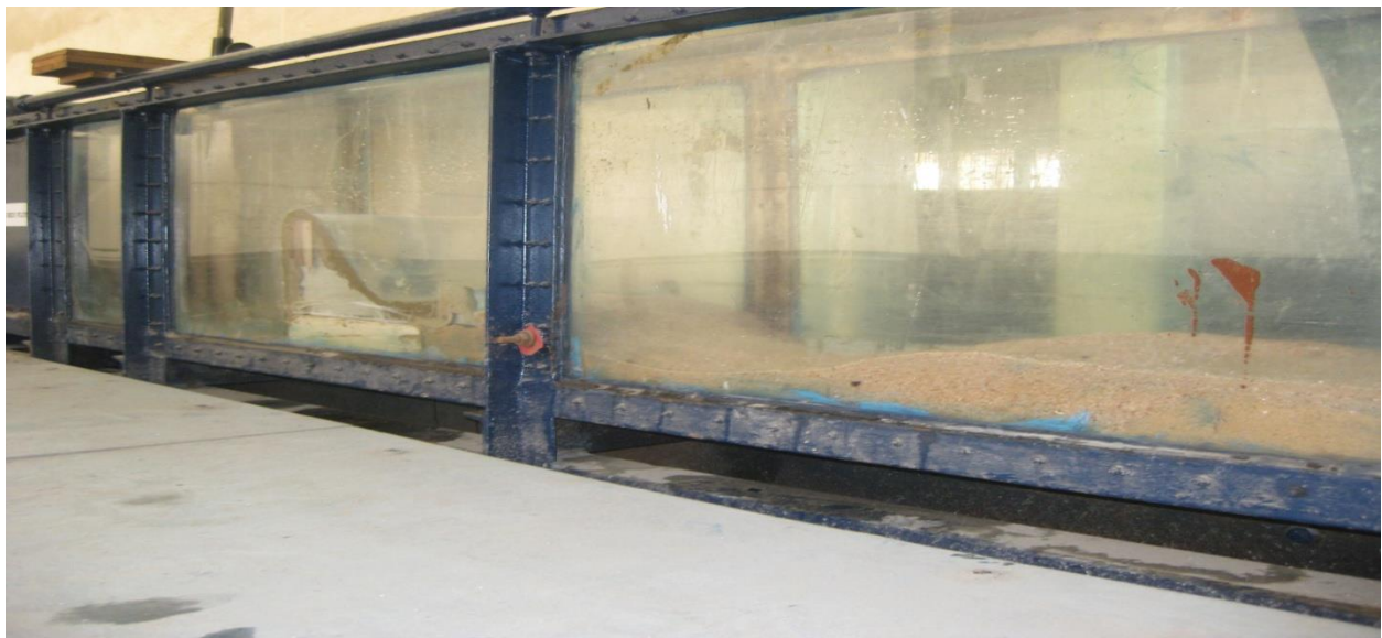
Figure 3.9: Scouring profile at downstream of ogee spillway with subsidiary dam with particle size 2.36mm on flat bed
