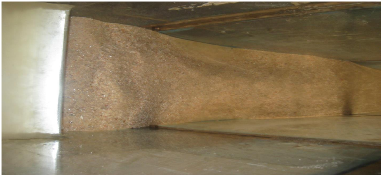
Figure 3.7: Scouring profile at downstream of ski jump bucket spillway with particle size 2.36mm on flat bed
