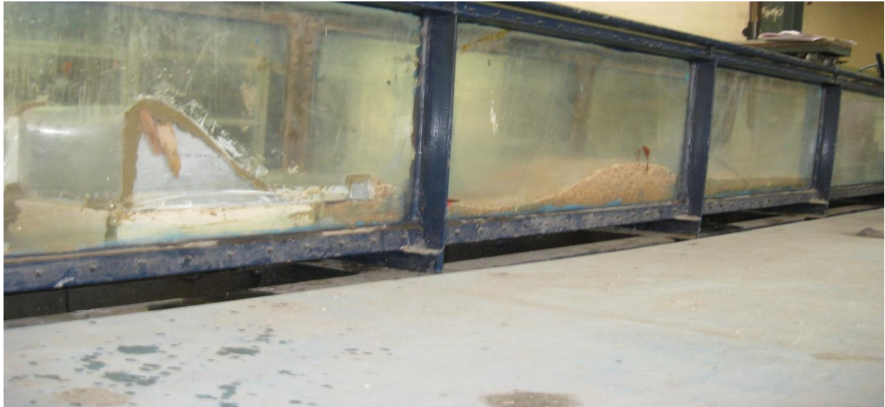
Figure 3.12: Scouring profile at downstream of ogee spillway with baffle wall with particle size 4.75mm on tilted bed (slope 1/300)
