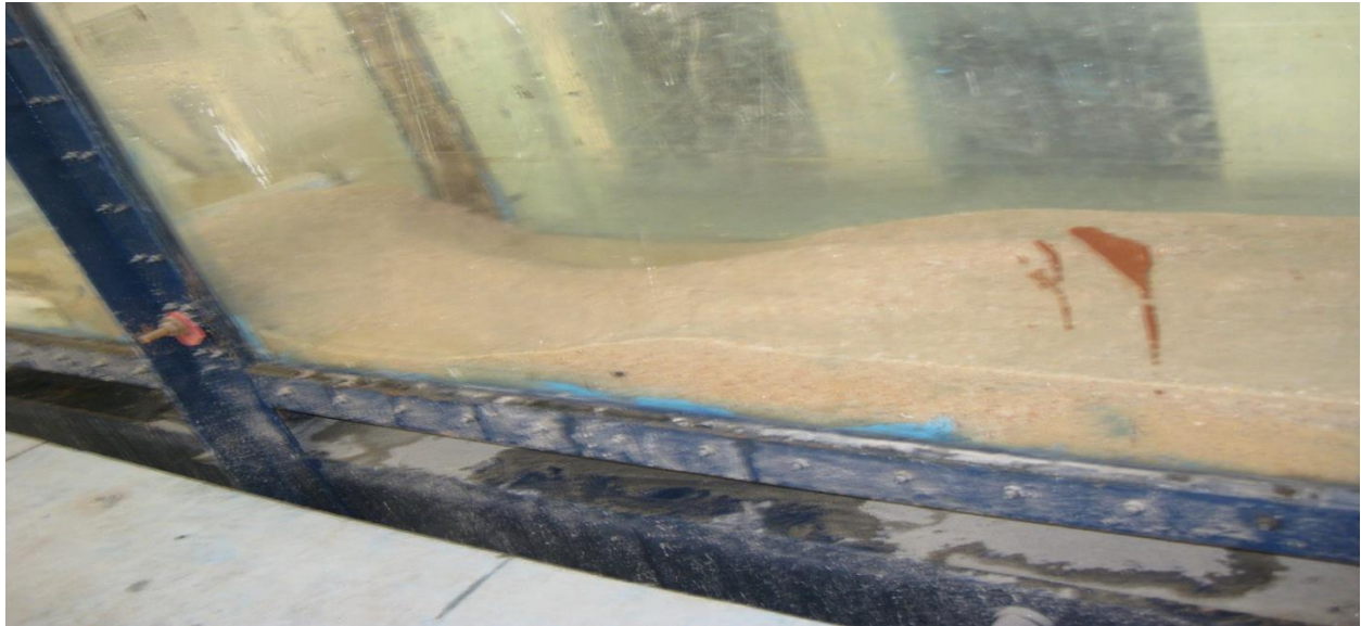
Figure 3.8: scouring profile at downstream of ogee spillway with subsidiary dam with particle size 2.36mm on tilted bed (slope 1/300)
