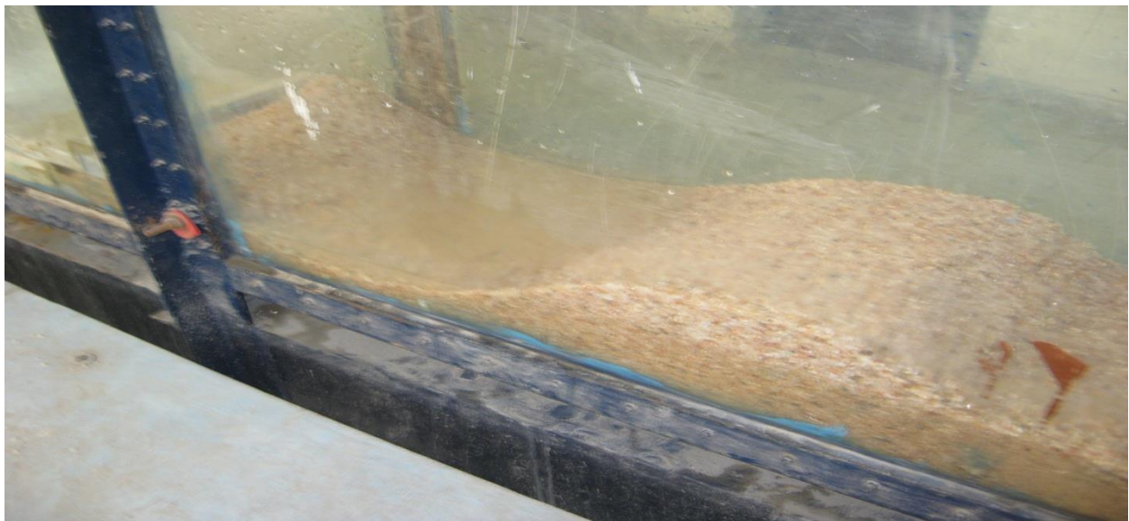
Figure 3.11: Scouring profile at downstream of ogee spillway with baffle wall with particle size 4.75mm on flat bed
