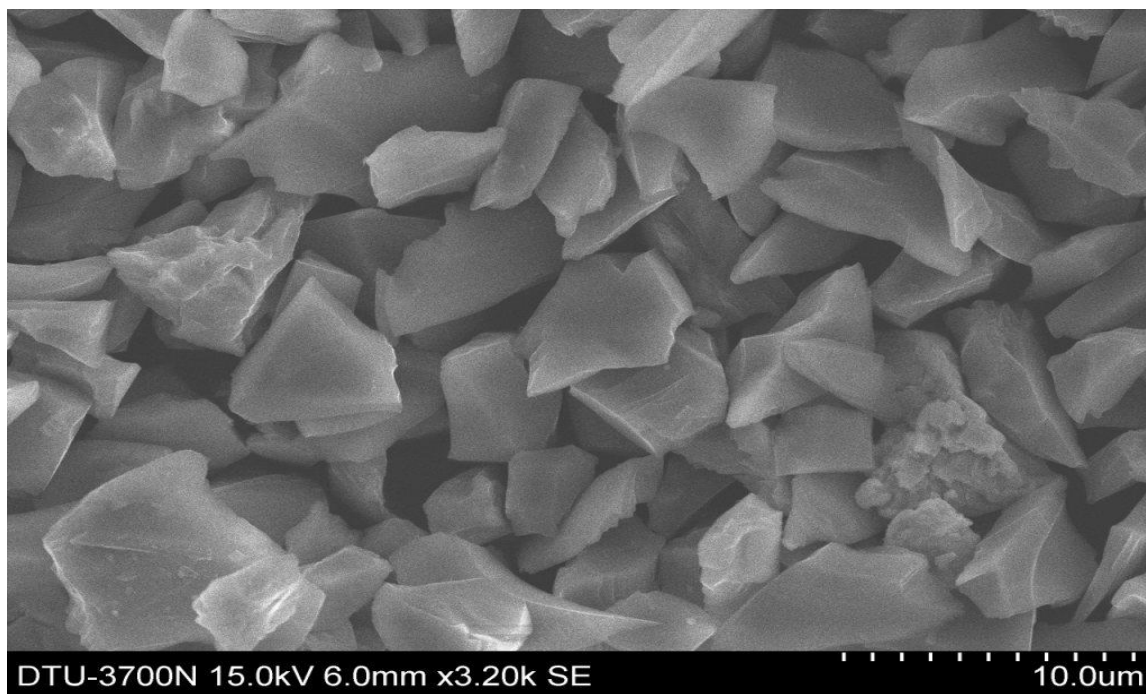
Fig. 4.5 showing the size of particles at 10 \mu\text{m} magnification
