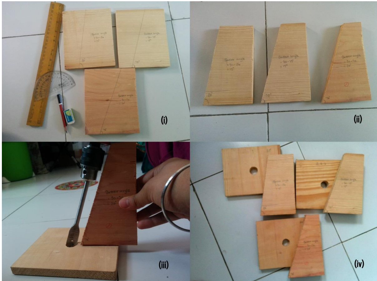
Fig4.4: Steps followed for achieving desired batter angle.
