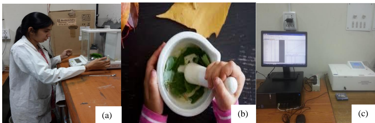
Figure 7. Weighing of sample (a); Grinding of leaves (b); Measurement of total chlorophyll content using spectrophotometer (c).
