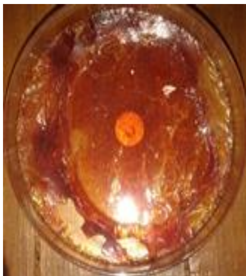
Figure 3.2.3: CdSe Nanoparticles Polyvinyl Alchohol film formed by in-situ method
