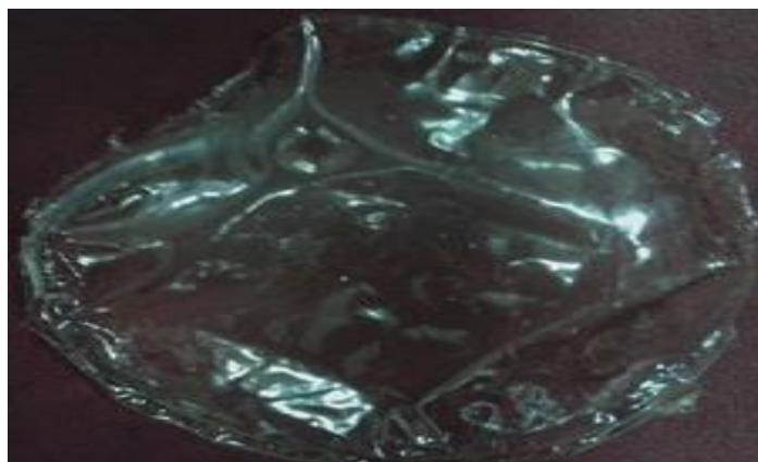
Figure 3.2.2CdSe nanoparticle PVA Film Synthesized by ex-situ method
