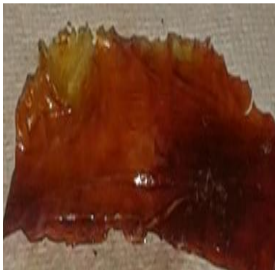
Figure 3.2.3: CdSe Nanoparticles Polyvinyl Alchohol film formed by in-situ method
