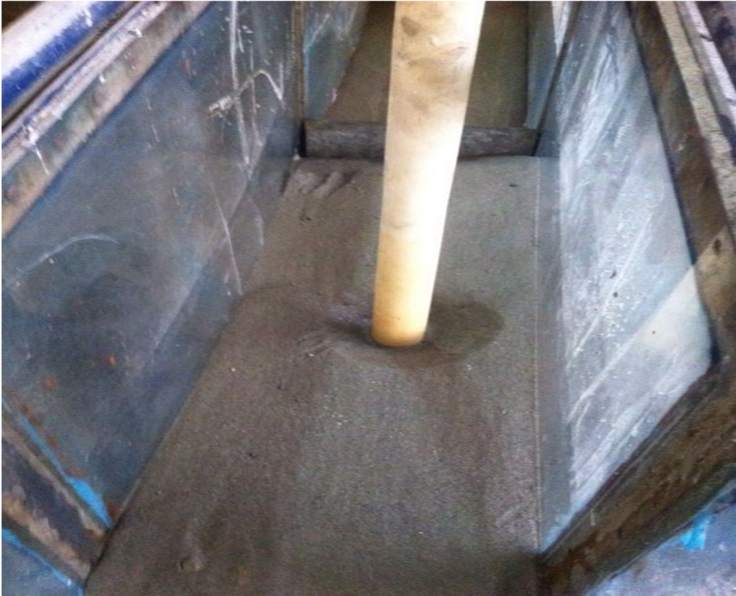
Figure 2 Scouring around the circular pier of diameter 5 cm
