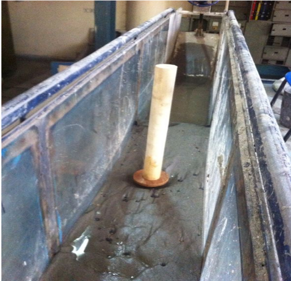
Figure 5 Scouring around the circular pier with circular collar of diameter 2.0D (D is diameter of circular pier)
