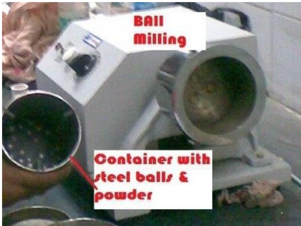
Fig. 3.12 Ball mill used for crushing of sintered pellets
