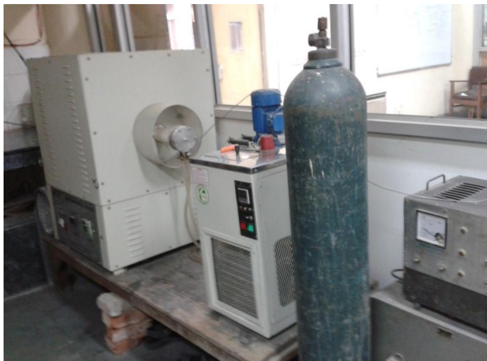
Fig.3.10 High temperature tube furnace
