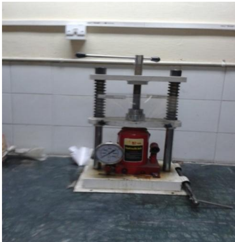
Fig. 3.3 Hydraulic jack machine used for pellets preparation
