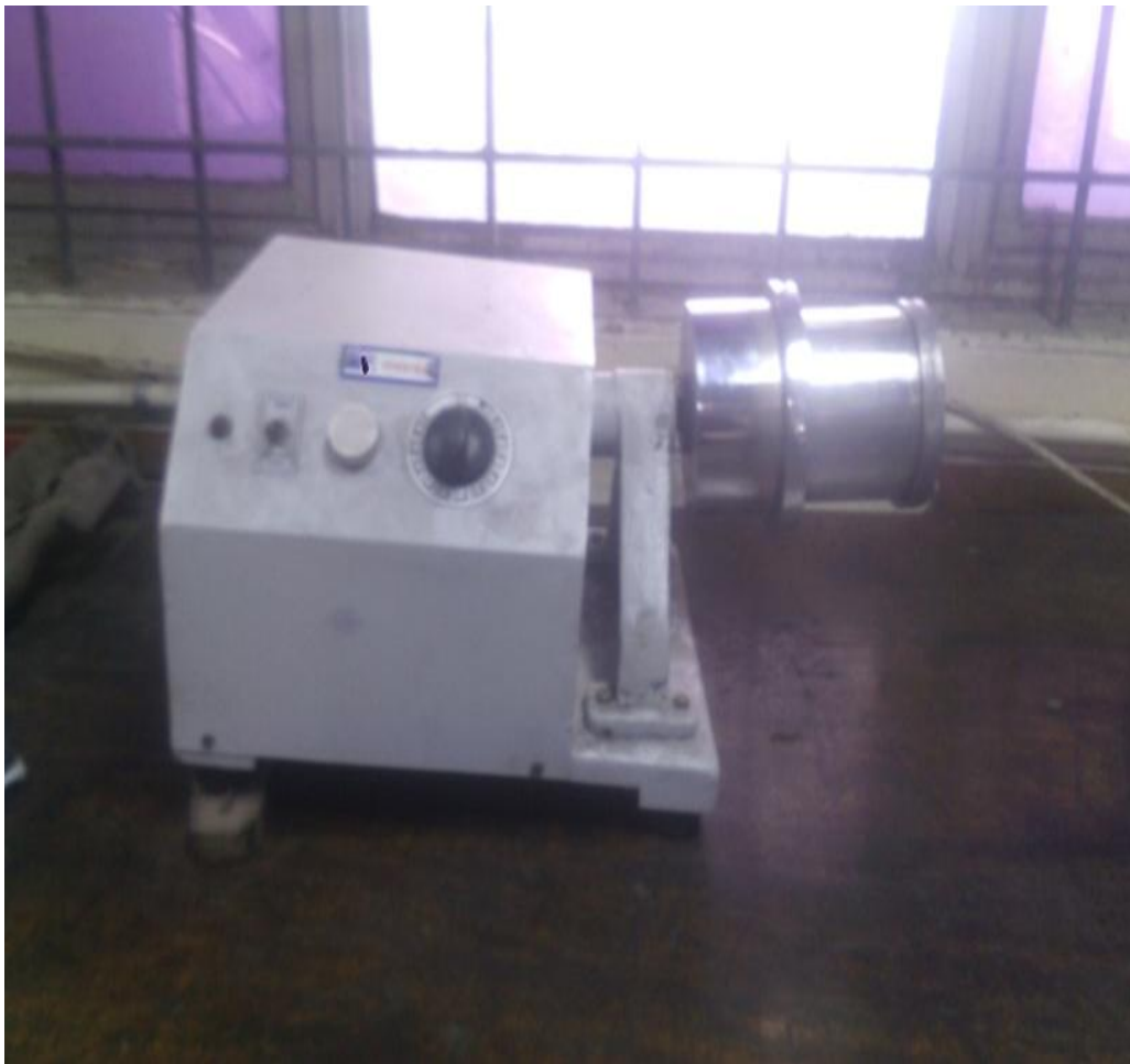
Fig.3.2 Ball mill used in present work
