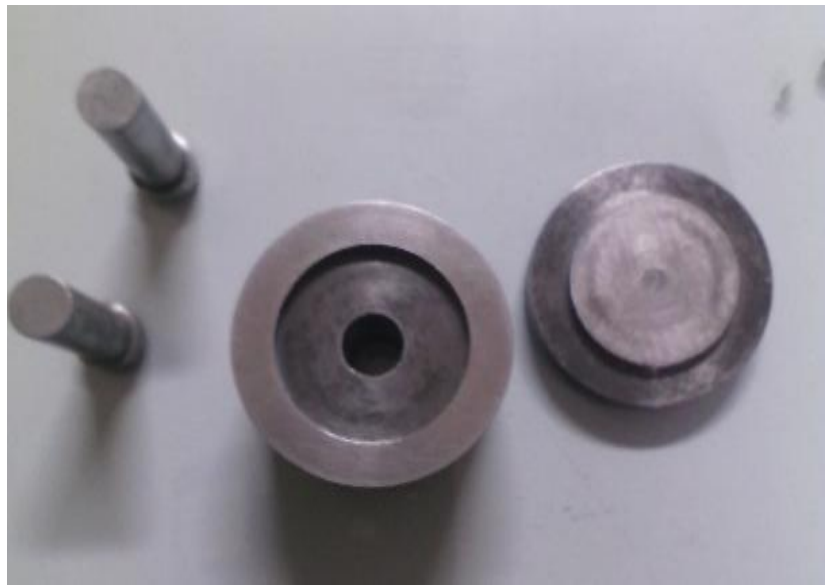
Fig. 3.4 Die used in pellet formation
