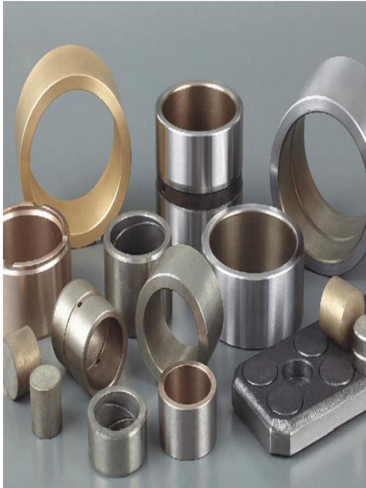
Fig. 1.7 Bearing production using PM
