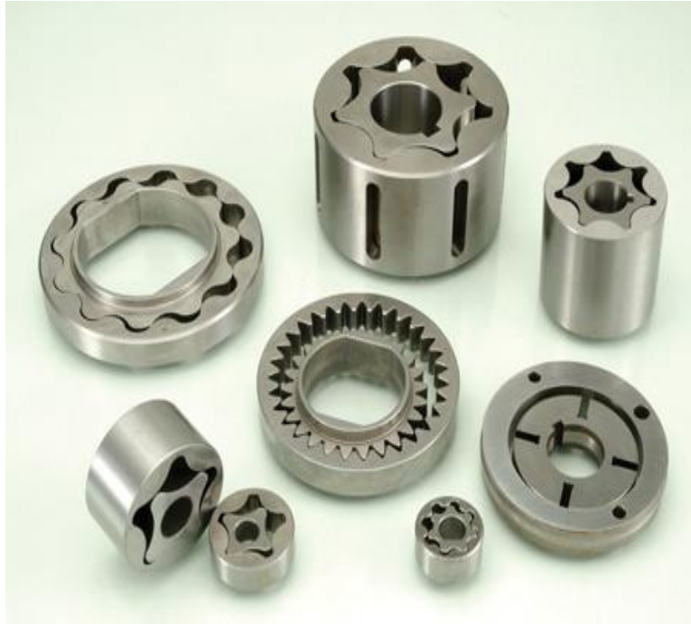
Fig. 1.5 Complex shapes manufactured by PM
