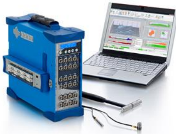
Figure 3.1: Experimental equipment (OROS 36) for vibration analysis.
