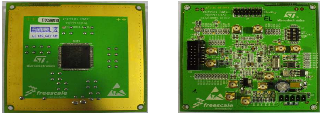
Figure 4.2: Placement of a DUT(IC) on PCB for EMC measurement.
