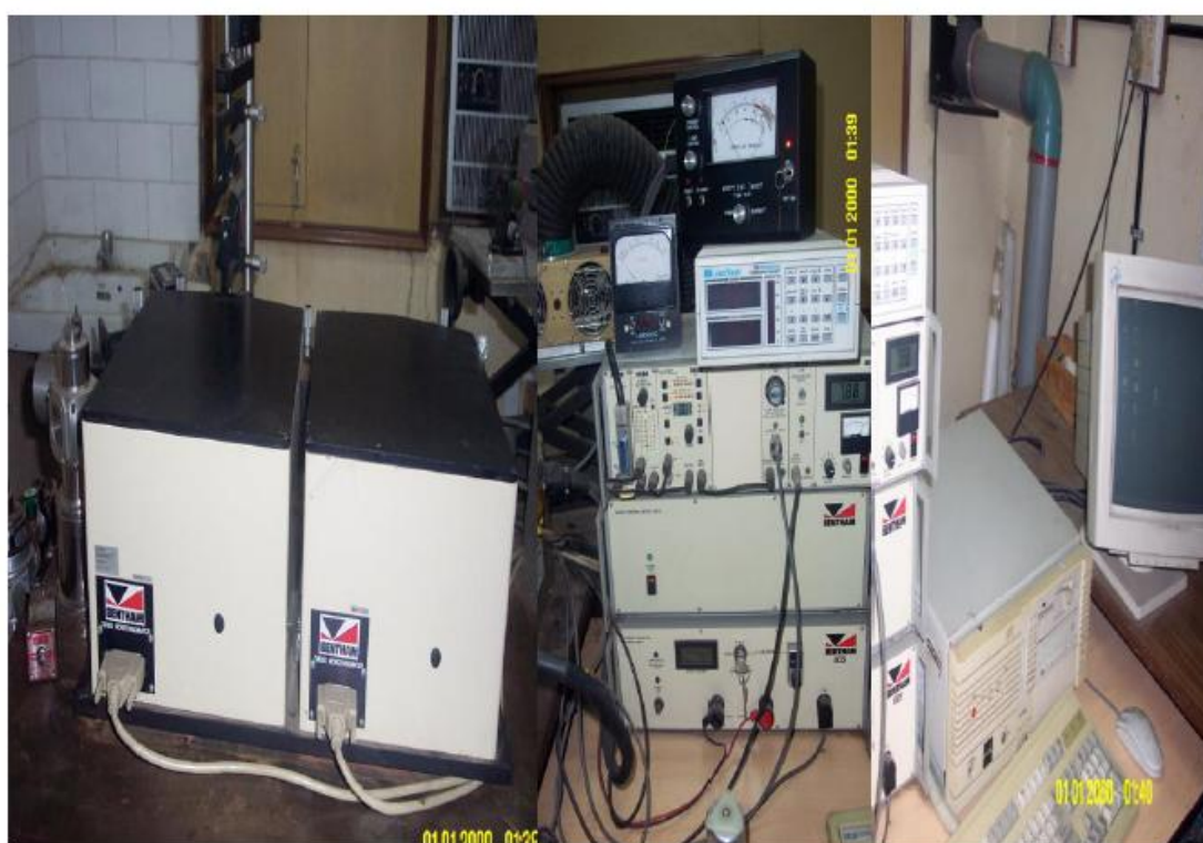
Figure 2.8 Home assembled PL system at NPL Delhi.
