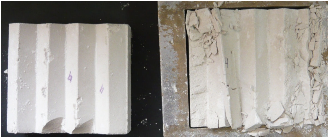
b) Sample of 30 degree asperity after shearing
