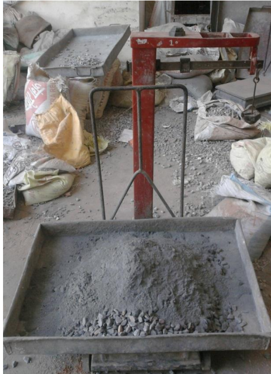
Fig-4.1.Weighing of batch of material for concrete mix
