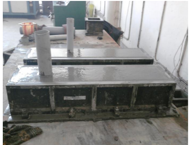
Fig-4.7. Casting of beams with Openings using PVC inserts
