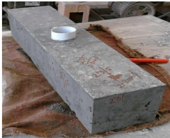
Fig.4.16. R.C.C Beam de-moulded, ready for curing
