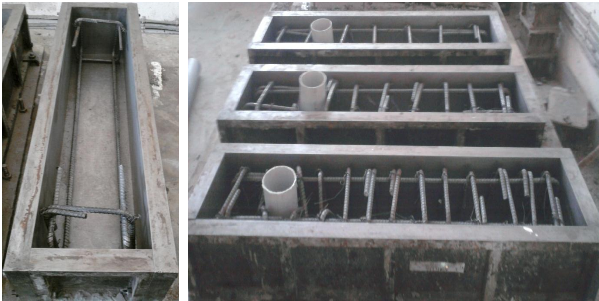
Fig-4.14. Beams ready to be cast (with & without shear reinforcements)
