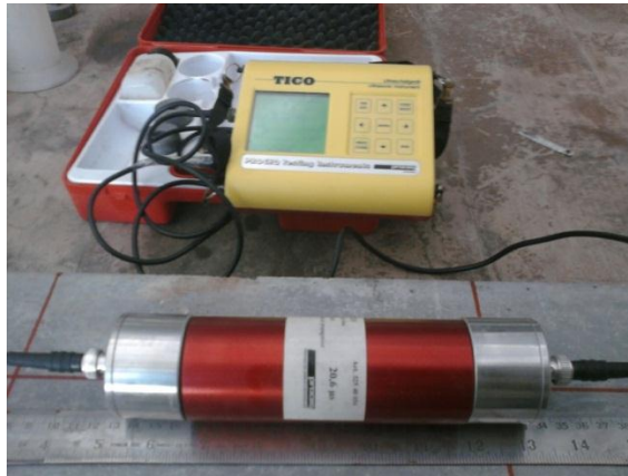
Fig.5.7. calibration using standard prism
