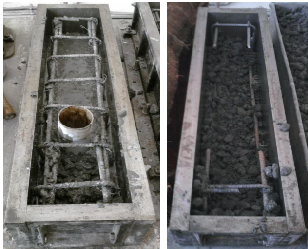
Fig.4.15.Casting of R.C.C beams
