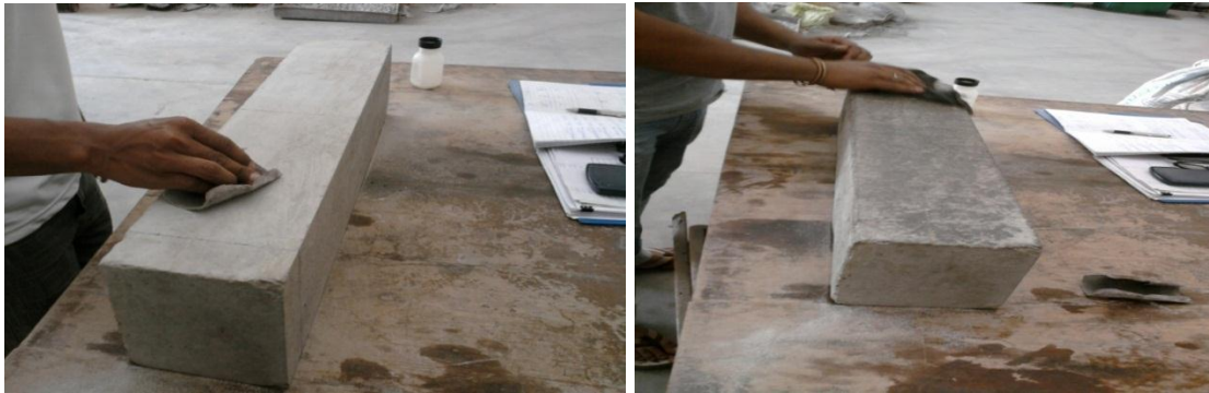
Fig5.2. Preparation of surfaces (Sanding & cleaning with damp cloth)
