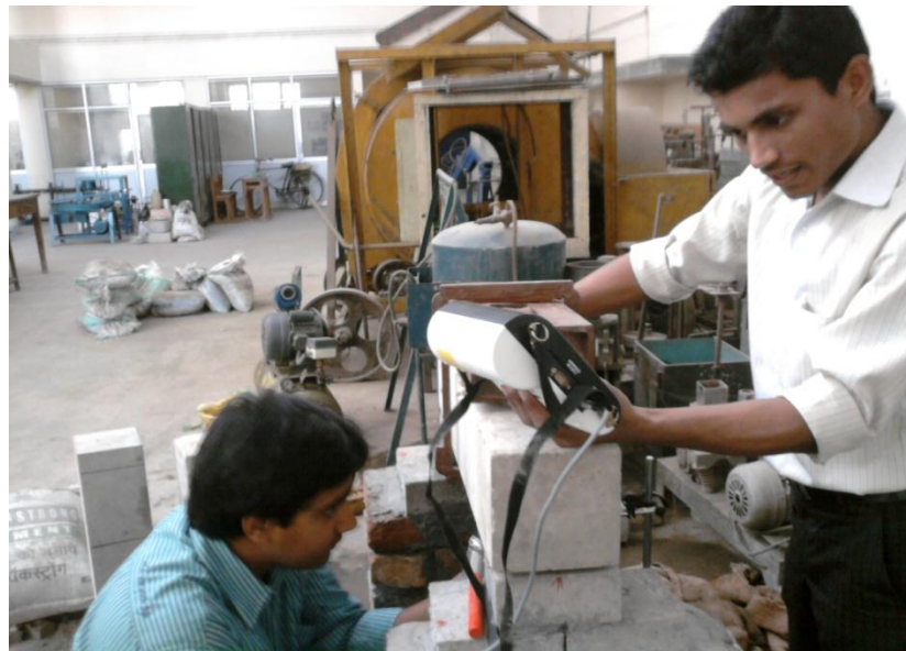
fig.5.12.Vertically upward R-H application
