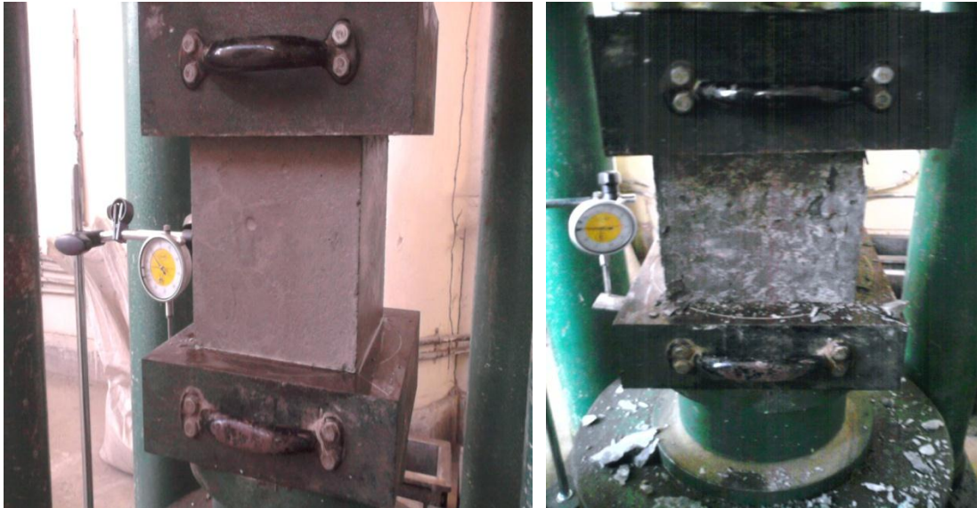
Fig.5.1. Compression Testing of Standard 15cm concrete cubes
