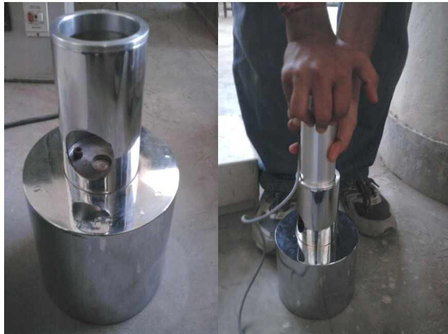
Fig.5.10.Rebound Hammer being calibrated on a 77 \pm 2 Anvil
