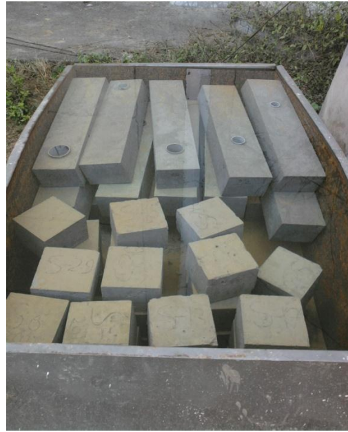
fig-4.9.All the specimens were cured for a period of 28 days in curing tanks
