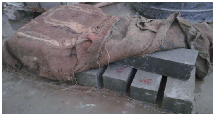
Fig.4.17.R.C.C beams under moist curing for 28 days
