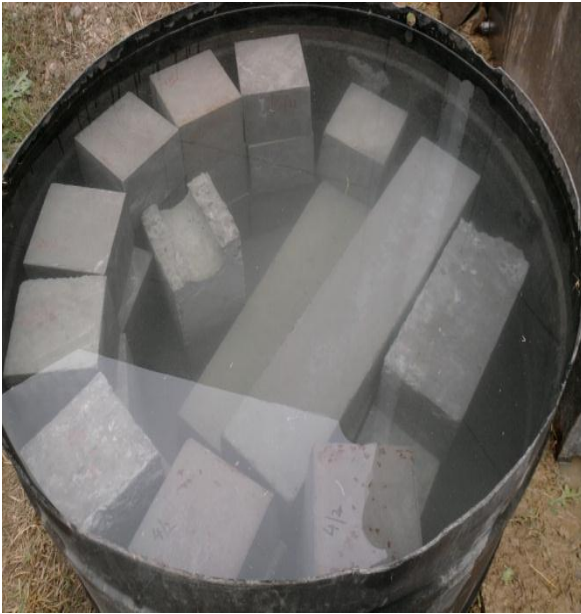
fig-4.9.All the specimens were cured for a period of 28 days in curing tanks
