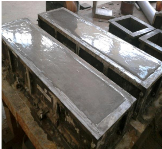
fig-4.6. Standard beam Specimen after casting (150mmx150mmx700mm)
