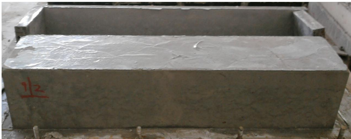
Fig-4.8. Demoulding of the Specimen.
