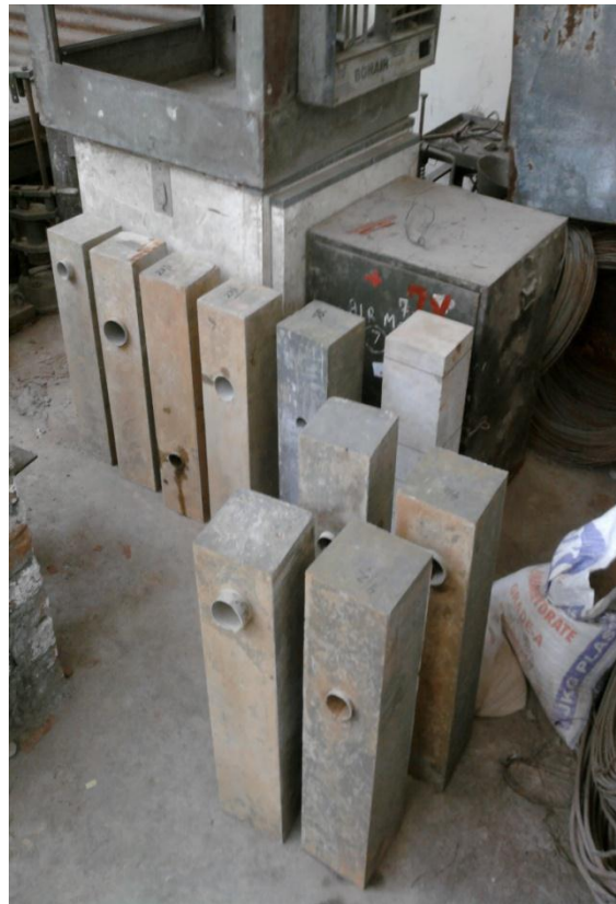
fig-4.10.Beams after 28 days of curing
