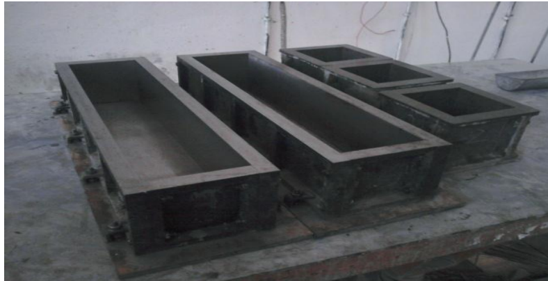
Fig-4.4. Clean & oiled standard beam & cube moulds for casting
