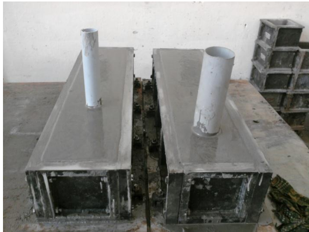
Fig-4.7. Casting of beams with Openings using PVC inserts
