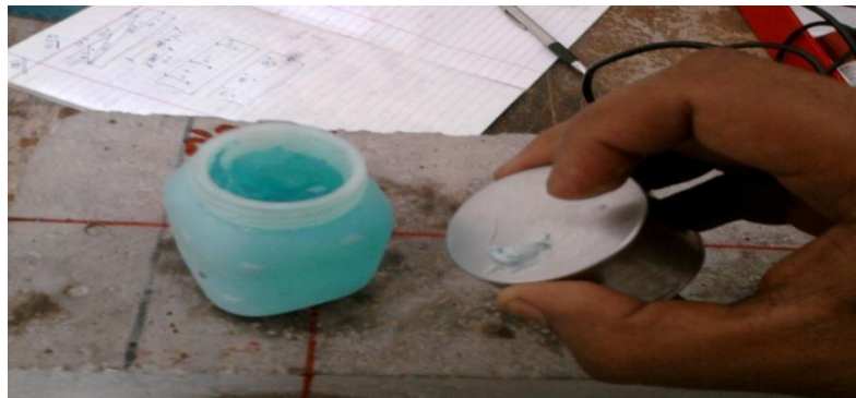
Fig.5.8. Application of Coupling Gel on the Transmitter & Receiver
