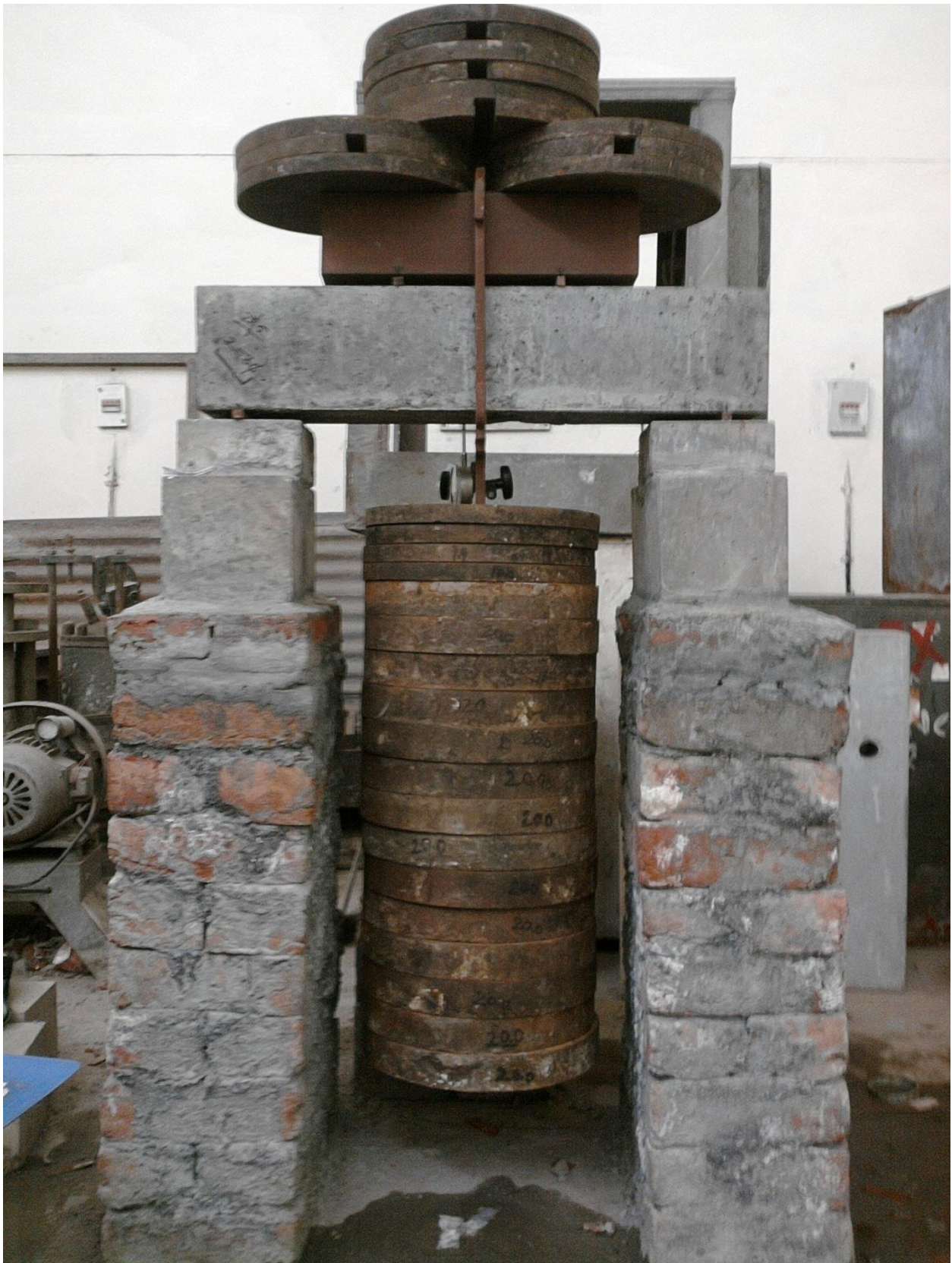
Fig.6.2.Apparatus to determine Load – Deflection Characteristics of Beams (Fully-Loaded)
