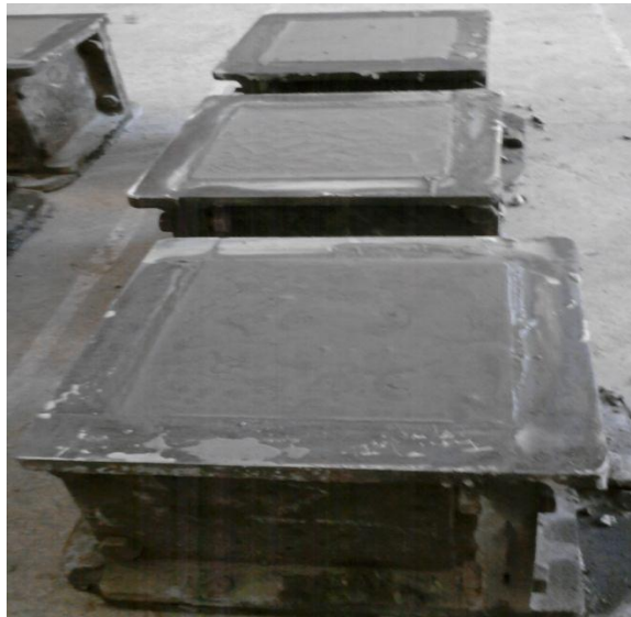
Fig-4.5. Standard cube after casting( 15cm)
