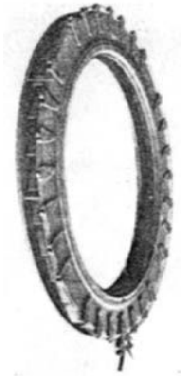
Fig.2.49 Guide blades ring with adjustable guide blades according to BBC.
